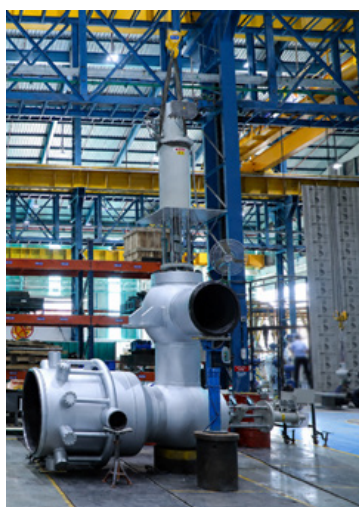
Figure 11: Stop and Control Dual Stem Turbine Bypass Valve
