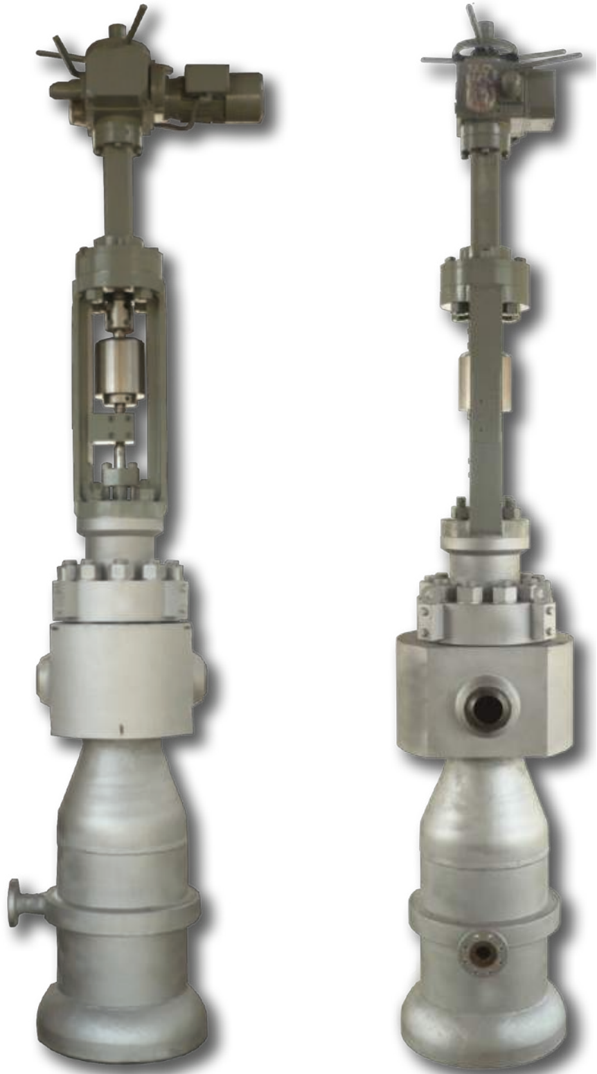
A custom VECTOR™ velocity control HP turbine bypass steam pressure-reducing valve with desuperheater for a power station in Eastern Europe featuring: two inlets and fast-stroking electric actuator, both as requested by the customer.
